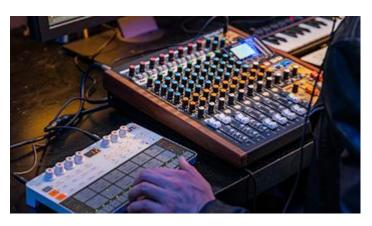
Standard MIDI input and output make it possible to use keyboards, drum machines, controllers, and other sources that employ MIDI technology with the Model 12. This also allows playbackstart commands to be triggered or external multi-track recorders and other external MIDI devices to be synchronized with the Model 12
